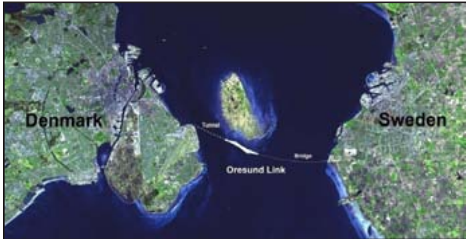
Figure B.1 Location and components of the Øresund Link (Image Source: NASA)
