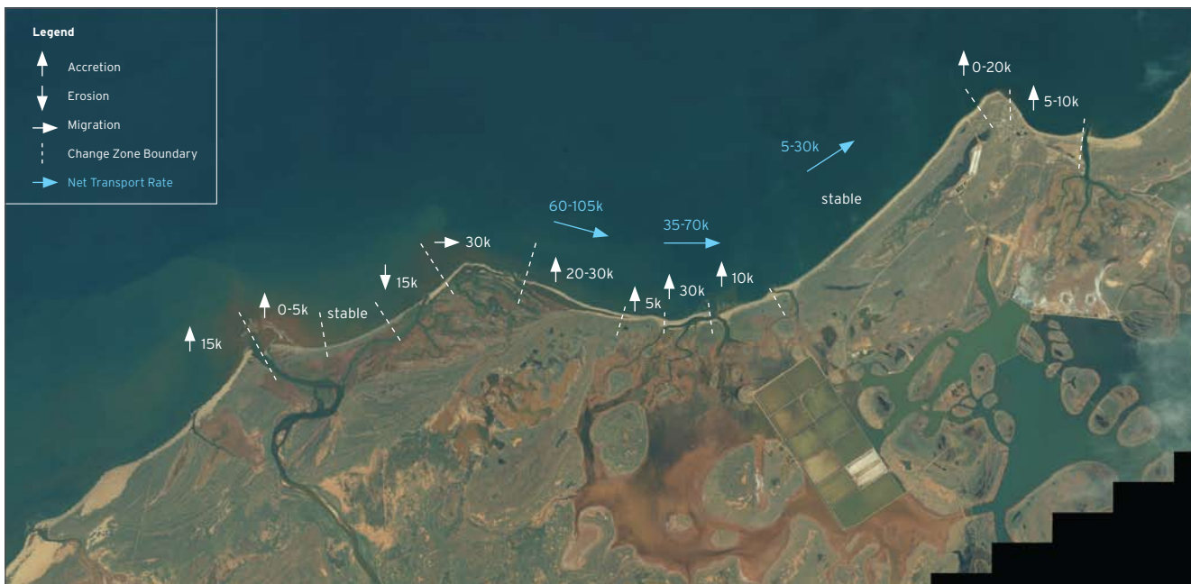
Figure 8.68: Erosion, Accretion and Net Transport Rates Derived from Shoreline Movements
